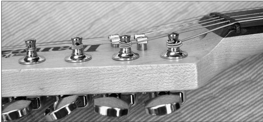
Figure 16-9: Coiling the string on the post.
