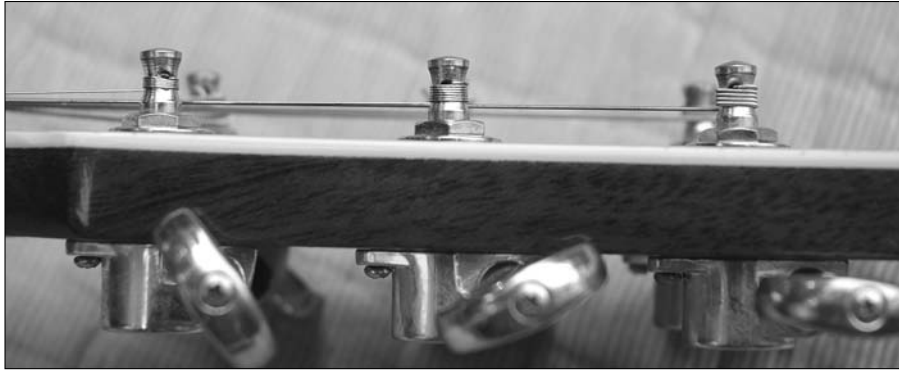
Figure 16-4: Coiling the string on the post.
